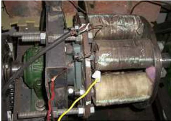
Fig. 3. energy-saving self-excitation electromagnetic retarding device
