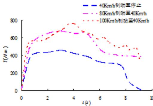
Fig. 4. variation curve of electromagnetic retarder torque with the braking time
